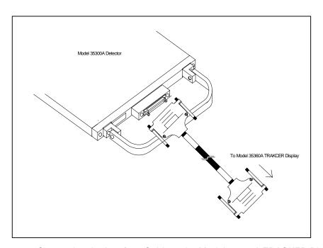
Figure 2-2. Connecting the Interface Cable to the Model 35360A TRACKER Display
